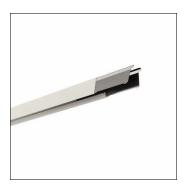
Licross®, trunking rail, of sheet steel, galvanised, coil coated, white, length: 4.500 mm, width: 64 mm, height: 67mm, through-wiring: 9x 2.5mm<sup>2</sup>, protection rating (complete): maximum IP64, depends on used inserts and accessories, insulation class (complete): insulation class I (protective earthing), certification: CE, UKCA, LABS conformity tested according to VDMA 24364:2018-05, packaging unit: 1 piece
