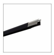
Licross®, trunking rail, of sheet steel, galvanised, coil coated, matt jet black (RAL 9005), length: 3.000 mm, width: 64 mm, height: 67mm, through-wiring: 9x 2.5mm², protection rating (complete): maximum IP64, depends on used inserts and accessories, insulation class (complete): insulation class I (protective earthing), certification: CE, UKCA, LABS conformity tested according to VDMA 24364:2018-05, packaging unit: 1 piece
