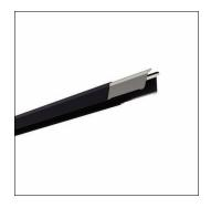
Licross, trunking rail, of sheet steel, galvanised, coil coated, matt jet black (RAL 9005), length: 3.000 mm, width: 64 mm, height: 67mm, through-wiring: 11x 2.5mm² (2x DALI, 1x emergency light), protection rating (complete): maximum IP64, depends on used inserts and accessories, insulation class (complete): insulation class I (protective earthing), certification: CE, UKCA, LABS conformity tested according to VDMA 24364:2018-05, packaging unit: 1 piece
