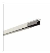
Licross<sup>®</sup>, trunking rail, of sheet steel, galvanised, coil coated, white, length: 3.000 mm, width: 64 mm, height: 67mm, through-wiring: 11x 2.5mm<sup>2</sup>, protection rating (complete): maximum IP64, depends on used inserts and accessories, insulation class (complete): insulation class I (protective earthing), certification: CE, UKCA, LABS conformity tested according to VDMA 24364:2018-05, packaging unit: 1 piece
