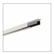
Licross®, trunking rail, of sheet steel, galvanised, coil coated, white, length: 1.500 mm, width: 64 mm, height: 67mm, through-wiring: 9x 2.5mm², protection rating (complete): maximum IP64, depends on used inserts and accessories, insulation class (complete): insulation class I (protective earthing), certification: CE, UKCA, LABS conformity tested according to VDMA 24364:2018-05, packaging unit: 1 piece
