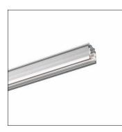
AX T, 3-phase track, installation type: suspended mounting, surface-mounted, mains connection: 220..240V/380..400V, AC, of extruded aluminium section, coated, grey, length: 3.000 mm, width: 32 mm, height: 33mm, protection rating (complete): IP20, insulation class (complete): insulation class I (protective earthing), certification: CE, ENEC, packaging unit: 1 piece
