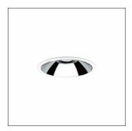
Lunis 21, XL, downlight, of PC, light emission: direct distribution, LED rated luminous flux: 3.360lm, light colour: 830, control gear: ECG, with terminal, 5-pole, mains connection: 220..240V, AC, housing, round, of diecast aluminium, traffic white (RAL 9016), diameter: 213mm, protection rating (complete): IP20, protection rating (on room side): IP54, insulation class (complete): insulation class II (safety insulation), certification: CE, impact resistance: IK02, packaging unit: 1 piece
