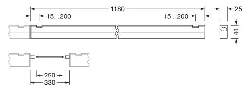
It is mandatory that the assembly instructions must be observed when planning and installing the electrical installation (to be found at www.siteco.com) Tolerances related to thermal, electrical and photometric data according to IEC 62722 Issued 09.04.2025 - Modifications and errors subject to change - Ensure that you always use the latest version -
