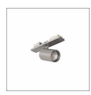
Licross<sup>®</sup> Spot 31, directional spotlight, light control with lens, of plastic, LED rated luminous flux: 5.140lm, light colour: 940, control gear: ECG, with plug, 3-pole, with phase selection, mains connection: 220..240V, AC, 50/60Hz, of aluminium, metallic grey (RAL 9006), length: 140mm, diameter: 90mm, protection rating (complete): IP20, insulation class (complete): insulation class I (protective earthing), certification: CE, packaging unit: 1 piece
