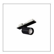
Licross® Spot 31, directional spotlight, light control with lens, of plastic, LED rated luminous flux: 5.190lm, light colour: 940, control gear: ECG, with plug, 3-pole, with phase selection, mains connection: 220..240V, AC, 50/60Hz, of aluminium, jet black (RAL 9005), length: 140mm, diameter: 90mm, protection rating (complete): IP20, insulation class (complete): insulation class I (protective earthing), certification: CE, packaging unit: 1 piece
