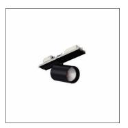
Licross® Spot 31, directional spotlight, light control with lens, of plastic, LED rated luminous flux: 3.680lm, light colour: 940, control gear: ECG, with plug, 3-pole, with phase selection, mains connection: 220..240V, AC, 50/60Hz, of aluminium, jet black (RAL 9005), length: 140mm, diameter: 90mm, protection rating (complete): IP20, insulation class (complete): insulation class I (protective earthing), certification: CE, packaging unit: 1 piece
