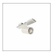
Licross® Spot 31, directional spotlight, light control with lens, of plastic, LED rated luminous flux: 3.680lm, light colour: 940, with plug, 3-pole, with phase selection, mains connection: 220..240V, AC, 50/60Hz, of aluminium, traffic white (RAL 9016), length: 140mm, diameter: 90mm, protection rating (complete): IP20, insulation class (complete): insulation class I (protective earthing), certification: CE, packaging unit: 1 piece
