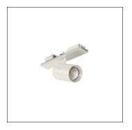
Licross® Spot 31, directional spotlight, light control with lens, of plastic, LED rated luminous flux: 3.650lm, light colour: 940, with plug, 5-pole, mains connection: 220..240V, AC, 50/60Hz, of aluminium, traffic white (RAL 9016), length: 140mm, diameter: 90mm, protection rating (complete): IP20, insulation class (complete): insulation class I (protective earthing), certification: CE, packaging unit: 1 piece
