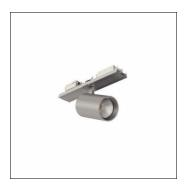
Licross® Spot 31, directional spotlight, light control with lens, of plastic, LED rated luminous flux: 3.680lm, light colour: 940, control gear: ECG DALI, with plug, 5-pole, mains connection: 220..240V, AC, 50/60Hz, of aluminium, metallic grey (RAL 9006), length: 140mm, diameter: 90mm, protection rating (complete): IP20, insulation class (complete): insulation class I (protective earthing), certification: CE, packaging unit: 1 piece
