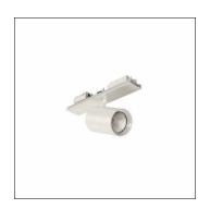
Licross<sup>®</sup> Spot 31, directional spotlight, light control with lens, of plastic, LED rated luminous flux: 5.140lm, light colour: 940, with plug, 5-pole, mains connection: 220..240V, AC, 50/60Hz, of aluminium, traffic white (RAL 9016), length: 140mm, diameter: 90mm, protection rating (complete): IP20, insulation class (complete): insulation class I (protective earthing), certification: CE, packaging unit: 1 piece
