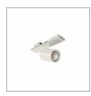
Licross<sup>®</sup> Spot 31, directional spotlight, light control with lens, of plastic, LED rated luminous flux: 5.250lm, light colour: 940, with plug, 3-pole, with phase selection, mains connection: 220..240V, AC, 50/60Hz, of aluminium, traffic white (RAL 9016), length: 140mm, diameter: 90mm, protection rating (complete): IP20, insulation class (complete): insulation class I (protective earthing), certification: CE, packaging unit: 1 piece
