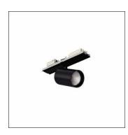
Licross<sup>®</sup> Spot 31, directional spotlight, light control with lens, of plastic, LED rated luminous flux: 5.140lm, light colour: 940, control gear: ECG DALI, with plug, 5-pole, mains connection: 220..240V, AC, 50/60Hz, of aluminium, jet black (RAL 9005), length: 140mm, diameter: 90mm, protection rating (complete): IP20, insulation class (complete): insulation class I (protective earthing), certification: CE, packaging unit: 1 piece
