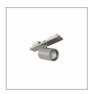
Licross<sup>®</sup> Spot 31, directional spotlight, light control with lens, of plastic, LED rated luminous flux: 3.650lm, light colour: 940, control gear: ECG DALI, with plug, 5-pole, mains connection: 220..240V, AC, 50/60Hz, of aluminium, metallic grey (RAL 9006), length: 140mm, diameter: 90mm, protection rating (complete): IP20, insulation class (complete): insulation class I (protective earthing), certification: CE, packaging unit: 1 piece
