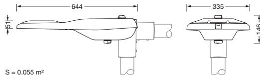
**Order No.: 5XE3B31Y08NB | GTIN (EAN): 4058352923825****Detailed technical description: SL21iQmd,ST0.5a,21550lm730,SR,D4i,LST,Za**
