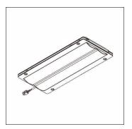
Streetlight 10 mini/midi, LED module, primary light control with pedestrian crossing, asymmetric right distribution, light distribution: PC-R, High Power LED, light colour: 750, colour temperature: 5000K, mains connection: 230..240V, 50Hz, LED module, length: 310mm, width: 137mm, height: 40mm, protection rating (complete): as luminaire, packaging unit: 1 piece
