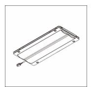
Streetlight 10 mini/midi, LED module, light distribution: ST1.2a, primary light characteristic: asymmetric, High Power LED, light colour: 722, colour temperature: 2200K, mains connection: 230..240V, 50Hz, LED module, length: 310mm, width: 137mm, height: 40mm, protection rating (complete): as luminaire, packaging unit: 1 piece
