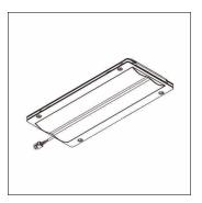
Streetlight 10 mini/midi, LED module, primary light control with pedestrian crossing, asymmetric left distribution, light distribution: PC-L, High Power LED, light colour: 730, colour temperature: 3000K, mains connection: 230..240V, 50Hz, LED module, length: 310mm, width: 137mm, height: 40mm, protection rating (complete): as luminaire, packaging unit: 1 piece
