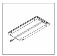
Streetlight 10 mini/midi, LED module, primary light control with pedestrian crossing, asymmetric right distribution, light distribution: PC-R, High Power LED, light colour: 730, colour temperature: 3000K, mains connection: 230..240V, 50Hz, LED module, length: 310mm, width: 137mm, height: 40mm, protection rating (complete): as luminaire, packaging unit: 1 piece
