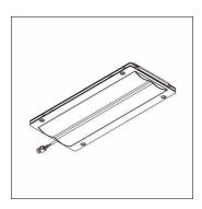
Streetlight 10 mini/midi, LED module, primary light control with cycle path optic, light distribution: P1.0a, primary light characteristic: asymmetric, High Power LED, light colour: 727, colour temperature: 2700K, mains connection: 230..240V, 50Hz, LED module, length: 310mm, width: 137mm, height: 40mm, protection rating (complete): as luminaire, packaging unit: 1 piece
