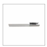
Modario<sup>®</sup> 31 connection compartment, white; connection compartment of sheet steel, galvanised, coated, with cable entry for four cables, Ø 8.5..13mm; 2x end cap 1x blank cover of PC/ABS, white; 1x connector of steel, galvanised, connector pre-assembled on trunking rail; dimension: (LxWxH) = 299 x 58 x 43mm; IP40; insulation class: insulation class I (protective earthing); certification: CE, UKCA; packaging unit: 1 piece
