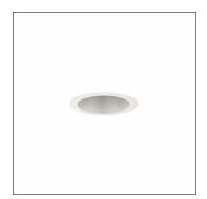
Lunis 31, -L, downlight, light control with reflector, light emission: direct distribution, LED rated luminous flux: 1.750lm, light colour: 840, mains connection: 220..240V, AC/DC, 0/50..60Hz, housing, of aluminium, white, protection rating (complete): IP20, protection rating (on room side): IP54, insulation class (complete): insulation class II (safety insulation), certification: CE, ENEC, packaging unit: 1 piece
