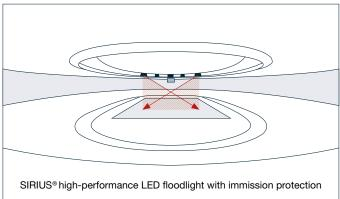
SIRIUS<sup>®</sup> enables highly targeted illumination of the required surface. There is no adverse impact on the surroundings and environment since scattered light is kept to a minimum.
