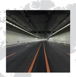
Zurich north bypass/Switzerland, 2017–2026 Interior zone lighting with continuous row luminaires Length: 11,600 m
