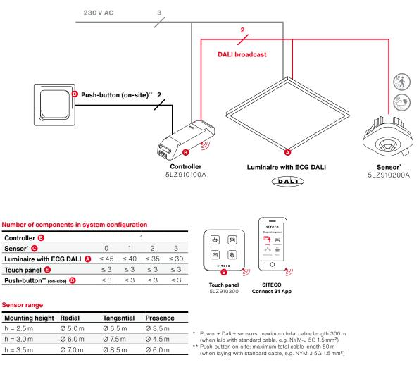
The above illustration serves only as an example of a circuit diagram for a light management system. For specific applications, individual planning (in particular for cable and circuit dimensioning, types of cables, fire barriers, routing, etc.) by qualified personnel is essential. Siteco GmbH assumes no liability for the correctness of the above illustration.
